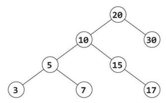
Commonly, we work with **binary search trees**. A binary search tree is a tree in which all nodes in the left subtree are less than the node's value, which is in turn less than the values of the all nodes in the right subtree. The above tree is a binary search tree.
